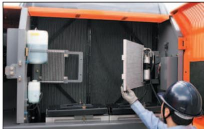
The oil cooler, radiator and intercooler are laid out in a parallel arrangement, instead of the conventional in-line arrangement. This parallel arrangement is significantly easier to clean around the engine. The air conditioner condenser can be opened for easy cleaning of the condenser and the radiator located behind.
