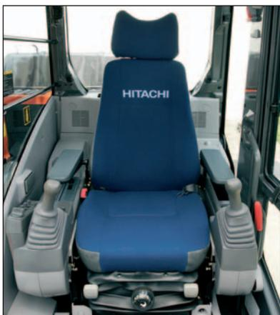
Wide adjustable armrests and a retractable seat belt are included. Short stroke levers mean fingertip control of hydraulics and allow for continuous operation with less fatigue. Three switches on the lever (optional) can be set to operate attachments other than buckets. The cab is pressurized to keep out dust. Noise and vibrations are kept to a minimum due to the elastic mounts, filled with silicone oil, the cab rests on.
